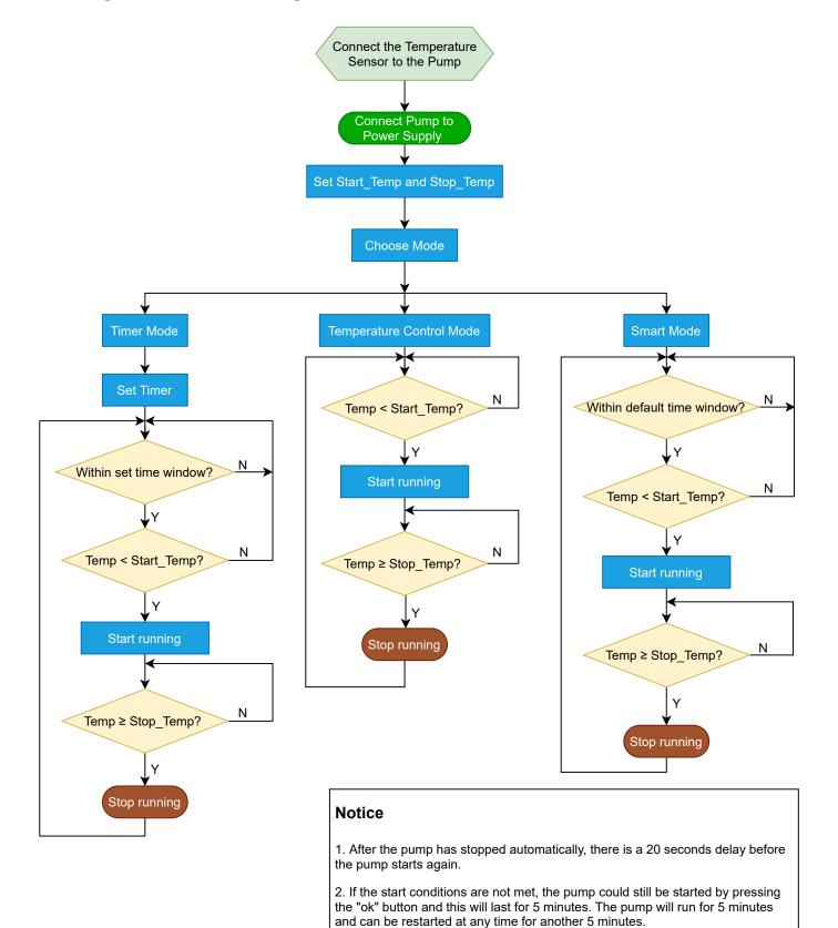
3. In Timer mode, the pump will run max. 30 minutes from the set starting time if
